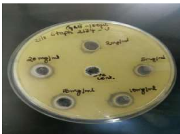
Figure 1: Showing the susceptibility of Staphylococcus aureus to varying concentrations of grape seed extract. The zones of inhibition is found to increase in size progressively to increased concentration of the extract.
